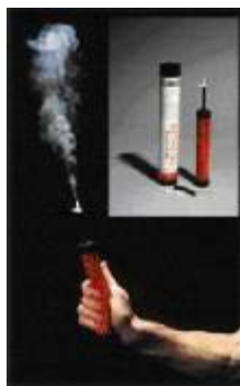
Figure 6: Smoke Pencil Used to Check for Air Leaks
